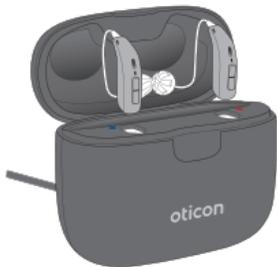
Place the hearing aids in the charging ports as shown in the picture and close the lid. Make sure that your hearing aids match the right and left color indicators on the charger's charging ports.
